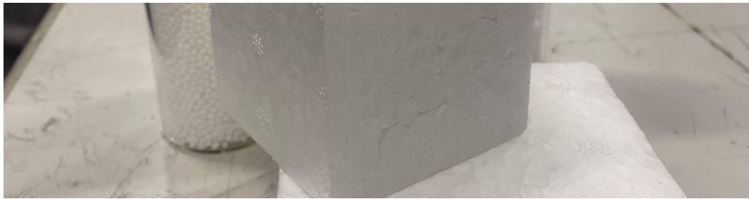
Fig. 6: Bio-based foamed beads for re-usable packaging and other consumer products. Source: Fraunhofer GmbH
