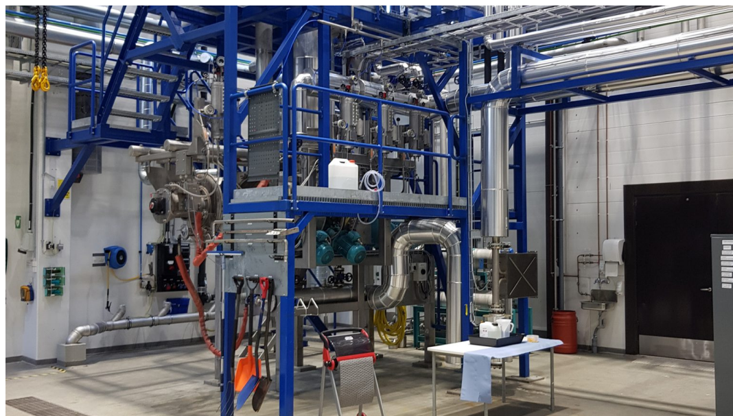
Fig. 3: Chemistry platform for scaling-up biopolymers. Source: VTT
